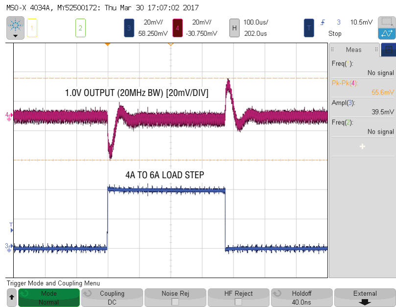
Figure 5. Measured Channel 1, 4A to 6A Load Transient ( V_{IN} = 12V , V_{OUT1} = 1.0V )
